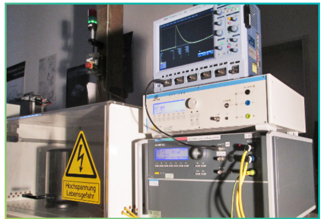
Test assembly: Surge and burst immunity test
